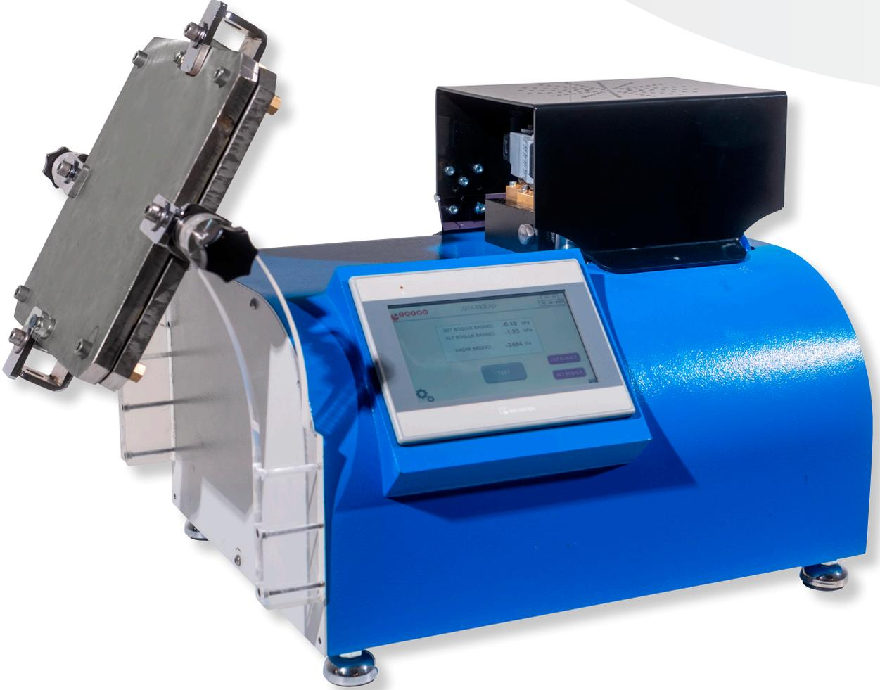
This device is used to measure the steady-state water permeability of geosynthetic barriers used to retain water in long-term applications. The test allows accurate measurement of water up to  $10^{-6} \text{ m}^3 / \text{m}^2 / \text{day}$
