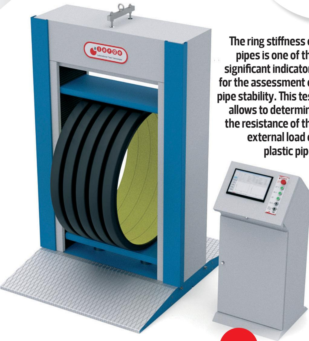
The ring stiffness of pipes is one of the significant indicators for the assessment of pipe stability. This test allows to determine the resistance of the external load of plastic pipe.
