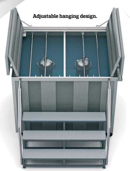
Internal pressure/hydrostatic tests are performed in conditioned water environment. Compliance with the standards **ISO 1167, ASTM D 1598, ASTM D 1599.** The water distribution into the AL TANK let ± 0,5 – 1 °C, provided by the circulation of water in the tank.
